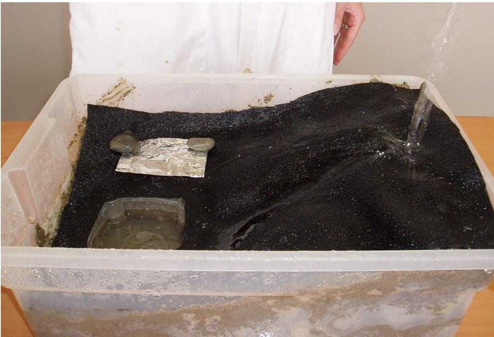
**Step B-2:** Use the watering can to pour water over the surface. Suggest that some students observe the sides of the container while others observe the surface. Draw attention to the *runoff, infiltration* and *percolation*.
