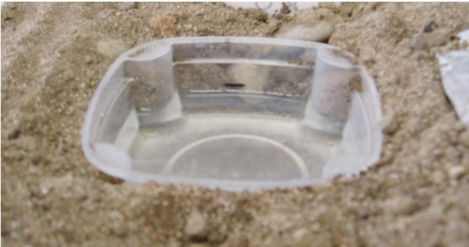
**Step A-3:** Make a few holes in the plastic container, this will allow water to flow out of the container, connecting it to the groundwater system. Draw a line at the half full mark and then place the plastic container at the bottom of the aquarium, or large tub, near the bottom of the slope. Build in the gravel around the container. This container is representative of a large water body such as a lake.
