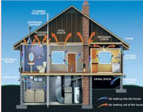
This photo shows areas where air enters and escapes homes
