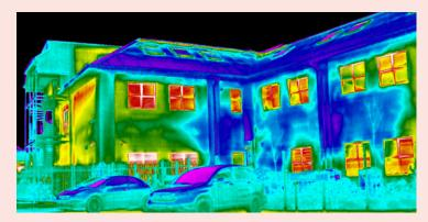
This is a thermogram, a photo taken using thermal infrared technology. Thermograms help identify areas of heat loss. Blue represents areas of low heat loss, and red and orange represent areas of high heat loss.
